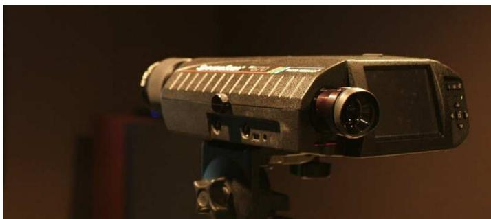
Figure 2 - Spectrophotometer used.
