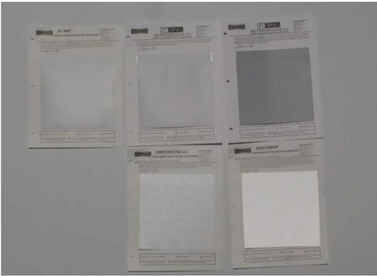
Figure 3 - Screen samples at 0 degrees from top left to right Da-Mat@, HD Progressive 0.9, HD Progressive 0.6, Video Spectra 1.5 and High Power on a Classic Cinema White background.
