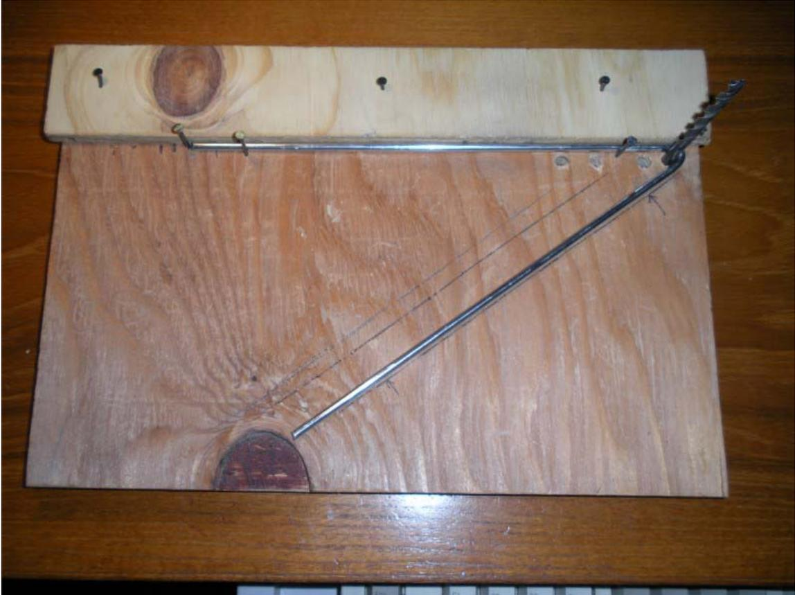
Referring to the photo, nail a small piece of plywood or other suitable material along one edge of a larger piece of plywood. Drill a 3/16-inch hole near one end of the plywood but away from it equal to the width of the welding rod so that when the shank of the drill is left in place as a pivot for the welding rod, the rod fits neatly between the drill and the plywood when it is bent.
