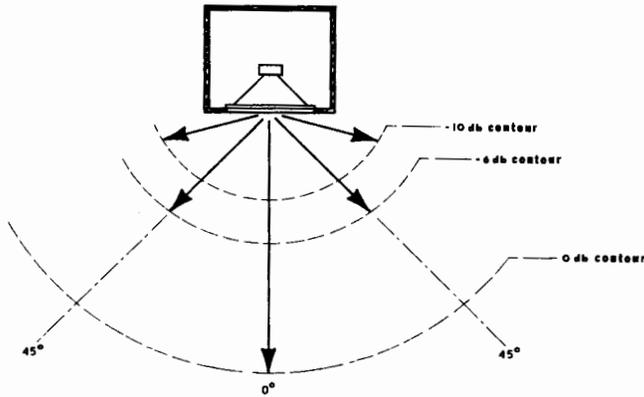
Fig. 1 Ideal Polar Response of a Loudspeaker.
