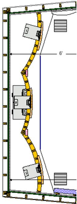
Figures 4 and 5: A curved speaker baffle wall
