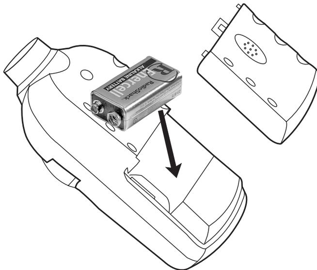
2. Place the battery in the compartment as indicated by the polarity symbols (+ and -) marked inside.
